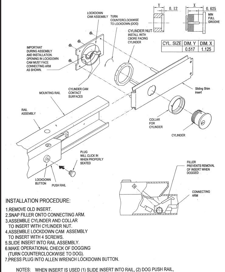
NOTES: WHEN INSERT IS USED (1) SLIDE INSERT INTO RAIL, (2) DOG PUSH RAIL,
