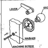
Drill a 3/8"(10mm) hole through door face as marked.insert machine screw from inside of door then tighten knob (or lever).
