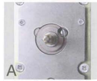
A. Remove Cover plate. Rotate the spindle either direction to expose and remove cylinder screws.
