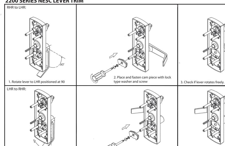
1. Rotate lever to LHR positioned at 90
