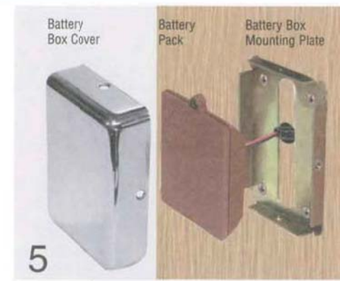
5. Connect battery pack and place inside of battery mounting plate. Position cover and fasten with three #6-32 x 5/16" screws.
