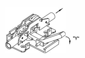
Press Lift Arm "Y" and ensure the direction before changing.
