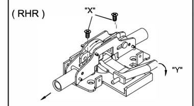
Fasten "X" at above screw hole position. Press Lift Arm "Y" to ensure the processing direction is reversed.
