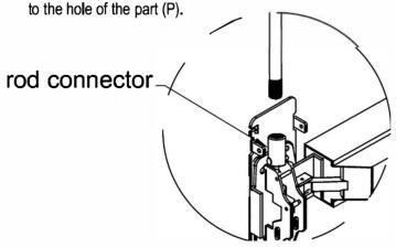
If top rod had been cut to fit door height, please drill hole for pin loading.
