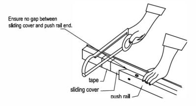
NOTE: the minimum length of the sliding cover must be 1"(25.4mm) or longer than length "C".
