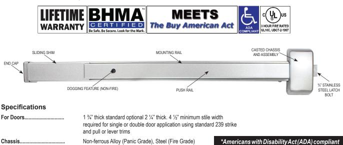
5 lbs opening force on ADA Series only Non-ferrous Alloy. Covers stock hollow metal doors \*Refer to the Price List for Stock Sizes and Finishes Furnished standard with wood and machine screws. Available with thru-bolts on request. Thru-bolts are standard Available, Prefix "NALRM" before MODEL # **Minimum Stile Requirements** Non handed, center hub, 2 <sup>3</sup>/<sub>4</sub>" backset
