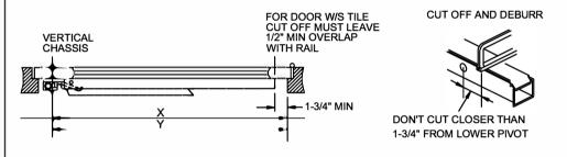
3. DEPRESS ARM INTO RAIL OPENING AND SLIDE RAIL ONTO CHASSIS. LEVEL RAIL AND FASTEN CHASSIS AND MOUNTING PLATE.
