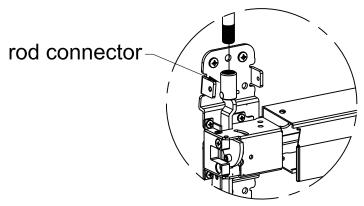
If top rod had been cut to fit door height, please drill hole for pin loading.
