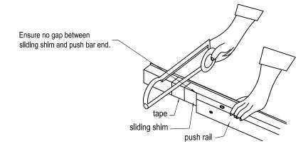
NOTE: the minimum length of the sliding shim must be 1"(25.4mm) or longer than length "C".
