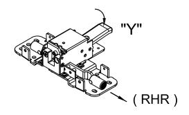
Press Lift Arm "Y" to ensure the processing direction is reversed.
