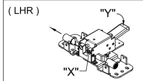
Press Lift Arm "Y" and ensure the direction before changing. The screw "X" is at the below hole position as figure shown
