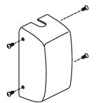
ATTACH COVER TO CHASSIS WITH (4) #8 TRUSS HEAD MACHINE SCREWS.
