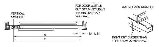
3. DEPRESS ARM INTO RAIL OPENING AND SLIDE RAIL ONTO CHASSIS. LEVEL RAIL AND FASTEN CHASSIS AND MOUNTING PLATE.
