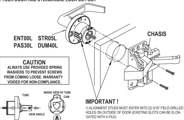
2) MAKE SURE TO TURN CAM CLOCKWISE BY PHILLIPS DRIVER HOLDING TUBE WITH FINGERS AS FAR AS IT WILL GO BEFORE RE-ASSEMBLING OF HANDLE TO PREVENT MIS-POSITIONING OF CAM. (SEE FIG. 1 AND FIG. 2)
