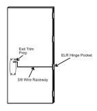
STEP 2: Run the wires from the ELR hinge through the 3/8" raceway starting at the ELR hinge & exiting into the pocket.
