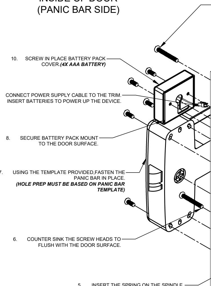
6. COUNTER SINK THE SCREW HEADS TO FLUSH WITH THE DOOR SURFACE.
