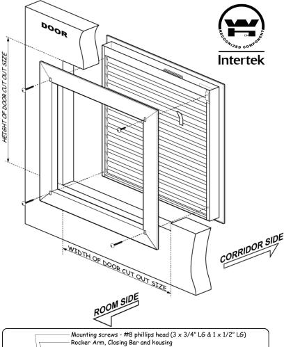
Mounting screws - #8 phillips head (3 x 3/4" L6 & 1 x 1/2" L6)
