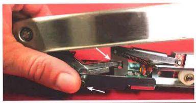
**6.** Using the allen wrench provided secure attaching kuckle.
