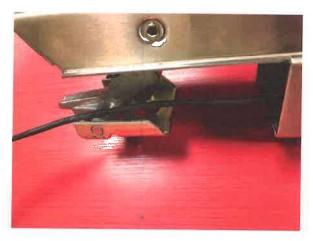
**9.** Add bracket #50453 to front activating bracket. Dropping it over the top and securing it with the screw provided.
