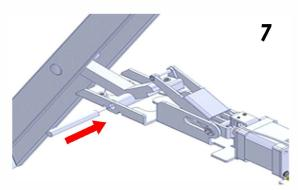
insert the Roll Pin through the holes to secure.
