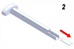
Flip over and remove the sliding shim cover.
