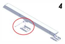
Remove the roll pin and separate the Push Rall from the Mount Base.
