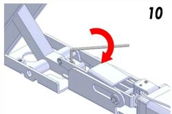
Fasten the stop screw in place using a Hex wrench.
