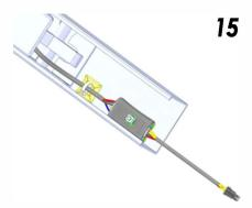
Stick the tie wire mount and use the cable tie to fix cable in place.
