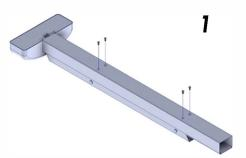
Flip over the device and remove fixed screws.
