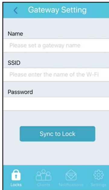
5. Set a name for your gateway, fill in the SSID and password for your wi-fi accordingly and tap **SYNC TO LOCK**
