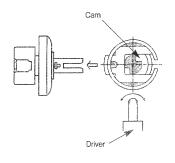
Make sure to turn cam anti - clockwise by driver as far as it will go before reassembling of cylinder to prevent mis-positioning of cam for classroom function.
