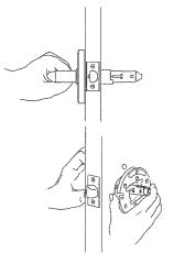
**CAUTION**: When using power screwdriver for installation, set to minimum torque setting.
