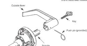
A. Insert key into cylinder. Insert push pin (or similar tool)
