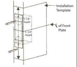
2. Mortise jamb according to measurement of installation template. Then fit strike and dust box into frame and secure into place with screws.
