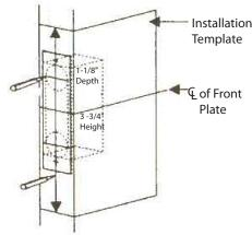
2. Mortise jamb according to measurement of installation template. Then fit strik and dust box into frame and secure into place with screws.
