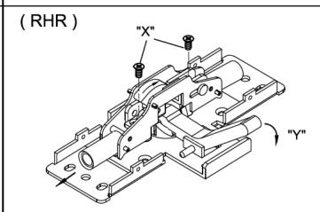
Fasten "X" at above screw hole position. Press Lift Arm "Y" to ensure the processing direction is reversed.
