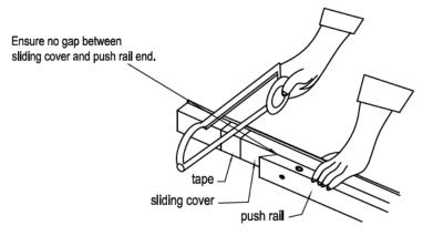
NOTE: the minimum length of the sliding cover must be 1"(25.4mm) or longer than length "C".
