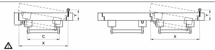
It may be the case that the panic fitting cannot be installed on extreme door situations according tostandard measurements
