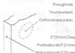
**C.** Drill the 2-1/8" (54mm) hole about halfway through door, then finish
