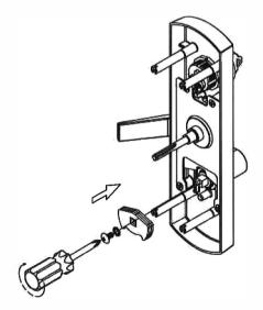
2.Place and fasten cam piece with locked type washer and screw
