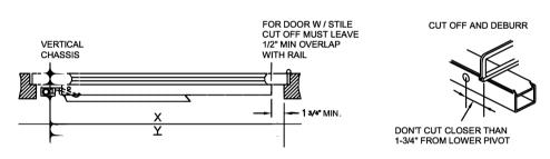
3. DEPRESS ARM INTO RAIL OPENING AND SLIDE RAIL ONTO CHASSIS. LEVEL RAIL AND FASTEN CHASSIS AND MOUNTING PLATE.
