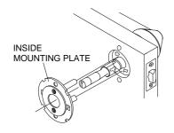
b. Press inside rose liner onto mounting plate and tighten mounting screws securely.
