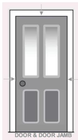
Seal gap between door and door jamb. Apply to Top part and both sides of the door jamb.
