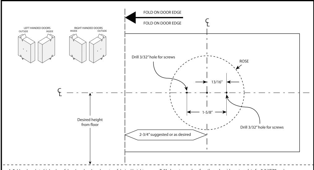
A. Fold and apply to high edge of door bevel and mark center of desired height from the floor.
