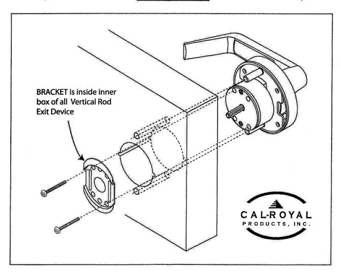
Bracket is packed with all VERTICAL ROD TYPE EXIT DEVICES inside each individual box. IT IS NOT PROVIDED WITH EXIT DEVICE TRIM.
