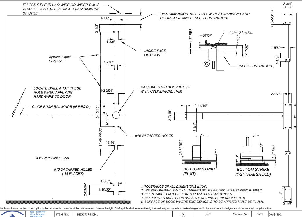
TO Tel.# (323) 888-6601 A L-R O Y A EDT-4130-12/25-1 of 1 **SCALE** FAX # (323) 888-6699 PRIMARY DIMENSION AF7760V SURFACE VERTICAL ROD FIRE RATED EXIT DEVICE BBT / ADG / CVL 07/29/2025 WEB SITE SHOWN IN INCHES CAL-ROYAL.COM PAGE 1 OF 1 REV: Ver-02
