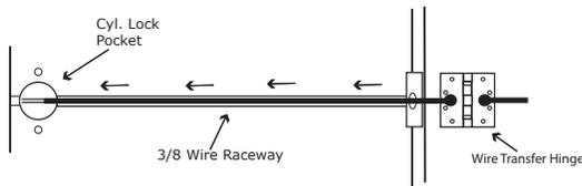
**STEP 3:** Screw the ETH hinge to the door. At this time **DO NOT** connect the hinge wires on the jamb side to the wires coming from the power supply.
