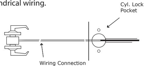
**STEP 6:** Carefully slip the connected cylindrical lock chassis into the lock pocket paying close attention not to pinch any wires.
